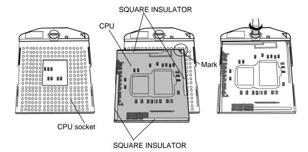
Figure 4-34 Installing the CPU
